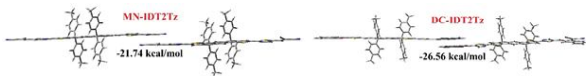
Figure 11. Intermolecular binding energies of dimer of MN-IDT2Tz and DC-IDT2Tz
