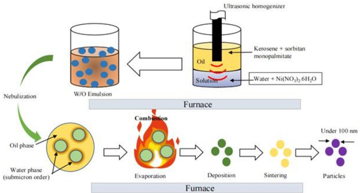
Figure 1: Thermal decomposition techniques to produce NiNPs<sup>66</sup>.
